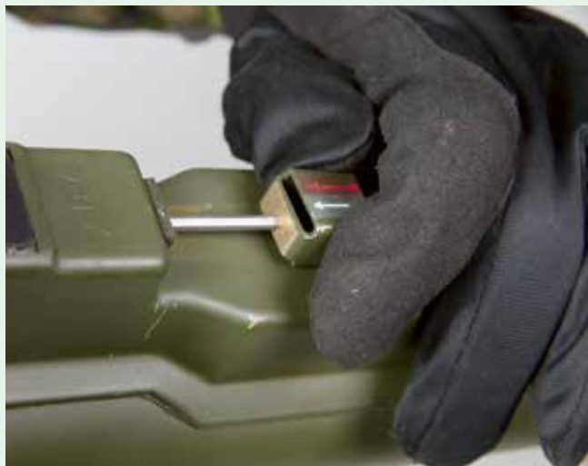
The trigger safety is removed by pushing it forward.
